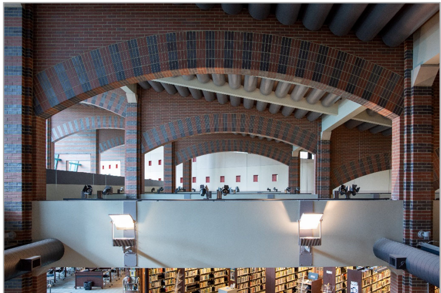
Left: Indirect Post Top Fixtures intended to spill some light onto ceiling and reflect most light back down to task plane
